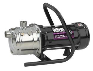
1" NPT suction and discharge threads, 3/4" garden hose adapter included, 180 feet of total dynamic head, maintains pressure up to 80 PSI Durable corrosion resistant construction Lift water as high as 25 feet and discharge pressures from 35 to 50 PSI 1 HP; max. flow rate is 720 Gallons Per Hour 520 GPH at 10 feet of discharge lift
