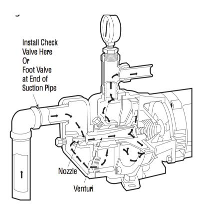
(Goulds Pumps) The Jet Assembly itself forms the suction chamber and the vacuum is created by the very high velocity of a stream of water passing through the jet. Basically, the jet assembly is composed of two parts. First, a nozzle which produces the high velocity stream of water.
